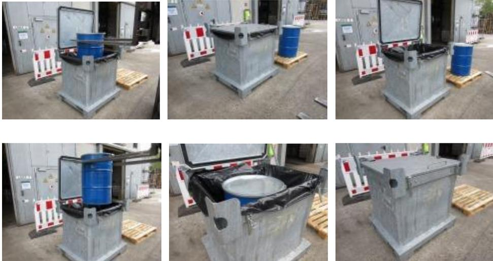
The IBC containers are not exclusively used for liquid waste (approved ADR packaging 31A) but are operated as salvage packagings under 11A (metal IBCs: steel containers for solids).
